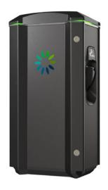
**Charging Mode** Mode 3 Socket (type 11) X 2 Socket or Tethered Lead AC Output Current (A) 6,10,16,20,25,32 3.7KW - 22KW Power outlet [kW] Rated voltage [V AC] 230 / 400 Frequency [Hz] 50 -25...+40 Temperature range [C] Degree of protection (IP) 44
